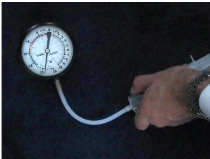
Fig. 3. A 60cc syringe can generate close to one atmosphere (30 in = 760 mm Hg) of negative pressure, dispelling the myth that syringe suction is “safer” than machine suction.
